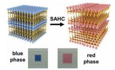
By taking advantage of a mechanochromic conjugated polydiacetylene (PDA) and the hydrocarbon-induced swelling properties of polydimethylsiloxane (PDMS), a sensor film that enables colorimetric differentiation among saturated aliphatic hydrocarbons (SAHCs) is developed. The unprecedented PDA-PDMS composite sensor undergoes a blue-to-red colorimetric transition that is dependent on the chain length of the hydrocarbon target.
