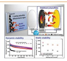
A bifunctional separator with a lightweight carbon-coating offers excellent dynamic electrochemical stability with Li-S cells: a high initial discharge capacity of 1389 mA h  $\rm g^{-1}$  and long cycle life. The static electrochemical stability is further evidenced by low self-discharge and excellent capacity retention after a 3 month rest period.
