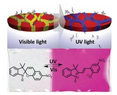
Photochromic membranes with reversible color switching and pronounced permeability change are created by incorporating spiropyran and spirooxazine derivatives into amphiphilic polymer co-networks. Truly tunable and responsive characteristics and the heterophase structure of the membranes are demonstrated to match the permeability properties of a given skin.
