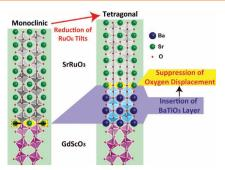
The manipulation of the displacement of the apical oxygen atom at the heterointerface is demonstrated as a tool to control the structural distortions that determine functional properties of transition-metal oxide thin films. High-resolution ABF-STEM imaging reveals that the interfacial octahedral connection angle is characterized by the picometer-order displacement of apical the oxygen atom. The findings provide a further degree of freedom for designing novel oxide-based heterostructures.
