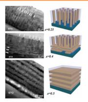
The precise tuning of inorganic nanocomposite thin films is realized using  $(YBa_2Cu_3O_{7-\delta})_{1-x}$ :  $(BaZrO_3)_x$  as a model system. A nanostructure switch from a vertical columnar structure to a horizontal multilayered structure is found with a transition, cross-ply structure at x = 0.4. Energetic considerations are used to explain the observed structures.
