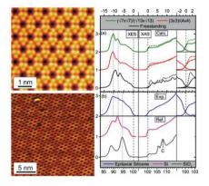
The electronic structure of epitaxial silicene monolayers on Ag(111) is explored through the complementary techniques of density functional theory (DFT) calculations and synchrotron-based soft X-ray spectroscopy experiments. Interaction with the underlying Ag substrate is found to confer a metallic nature upon the silicene monolayers, ruling them out as possible Dirac cone hosts.
